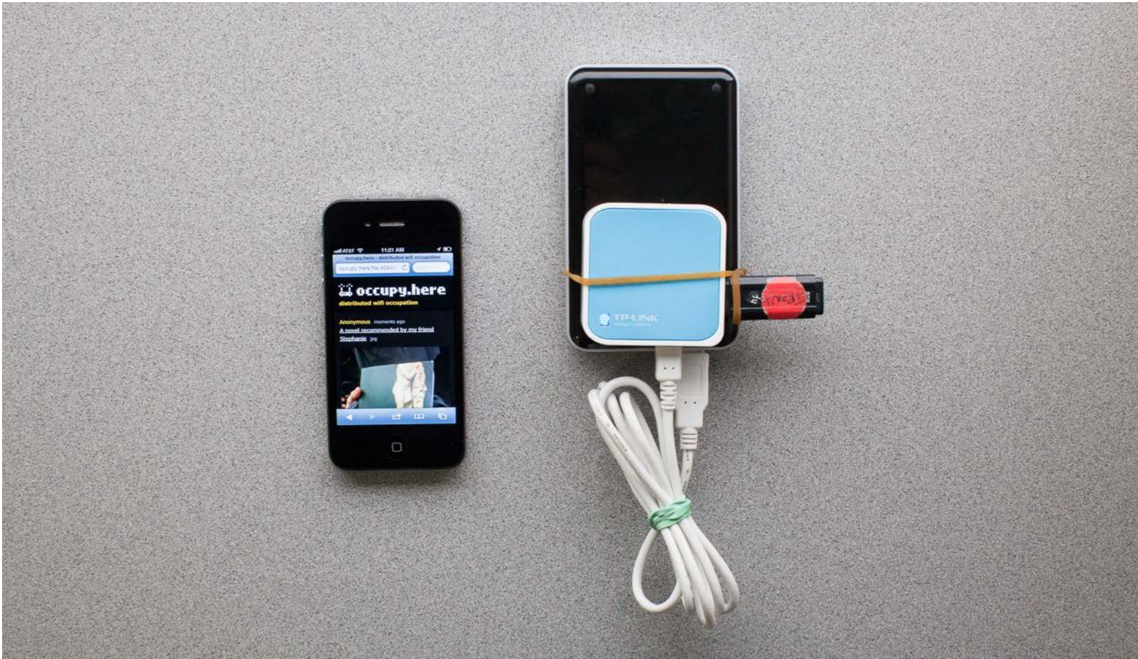
Occupy,here, a router that establishes a local area network from any mobile device. Created by Dan Phiffer in parallel with the Occupy movement.
